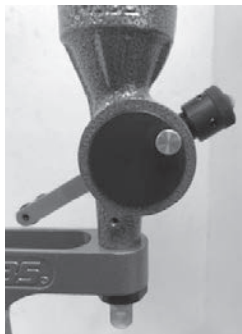
Cylinder position when setting for lightest load
